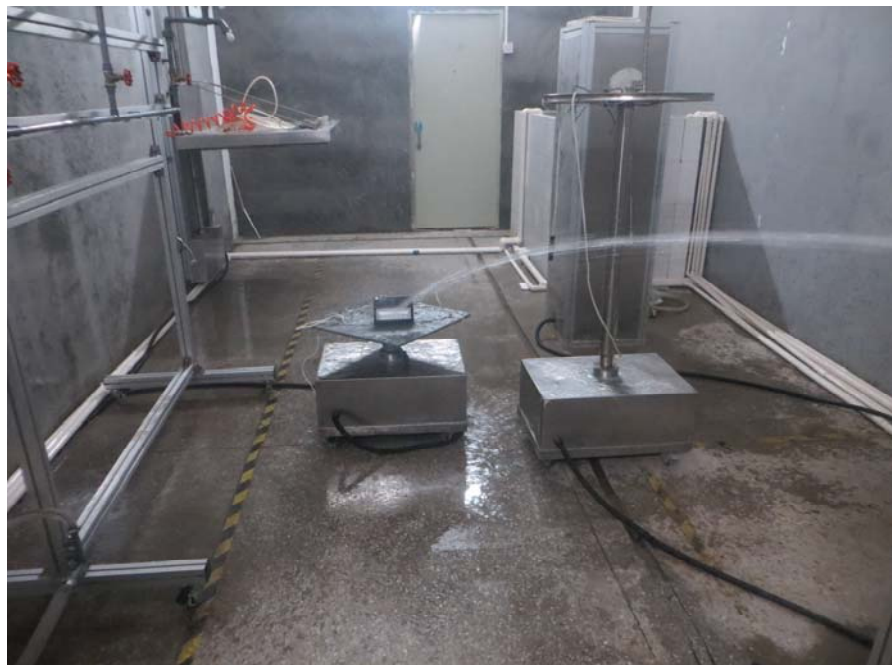
Figure 2 (IPX5 test photo)
